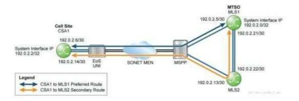
You wish to configure a secondary static route on MLS1 targeting the CSA1 system interface. The route must forward packets over the secondary route path as shown in the diagram. Given the following:
