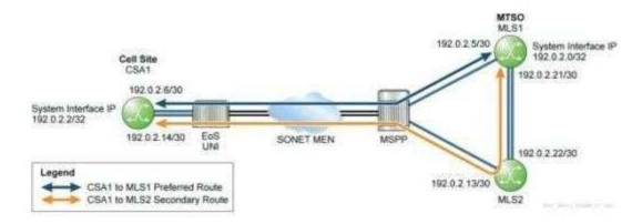
You must configure Label Distribution Protocol (LDP)-sync on the CSA1-to-MLS1 preferred static route. The route must forward packets over the preferred route path as show in the diagram. Given the following:
