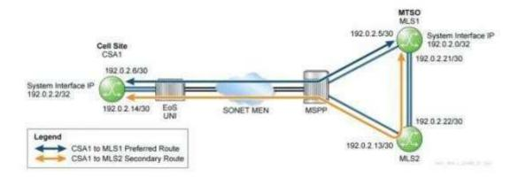
You wish to configure a preferred and a secondary static route on CSA1. targeting the MLS1 system interface. The preferred route must forward packets over the preferred route path as shown in the diagram. Given the following:
