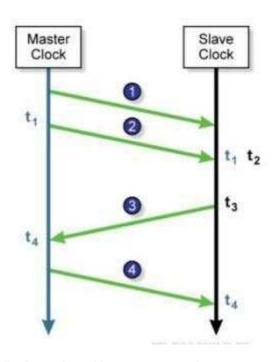
Each numbered item, 1, 2, 3, and 4, represents a message exchanged between an IEEE 1588v2/Precision Time Protocol (PTP) v2 master and slave.
