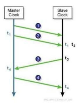
Each numbered item, 1, 2, 3, and 4, represents a message exchanged between an IEEE 1588v2/Precision Time Protocol (PTP) v2 master and slave. With which message does the master pass its t1 timestamp to the slave clock at item 2?
