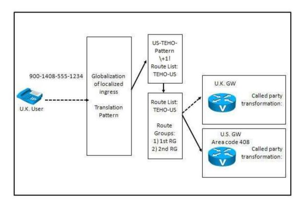
The exhibit shows centralized Cisco Unified Communications Manager configuration components for TEHO calls to U.S. area code 408 from the U.K. The PSTN access code for the U.K. is 9 and 001 for international calls to the U.S. Assuming the PSTN does not accept globalized numbers with + prefix. What should the Called Party Transformation Pattern at the U.S. gateway be configured as?
