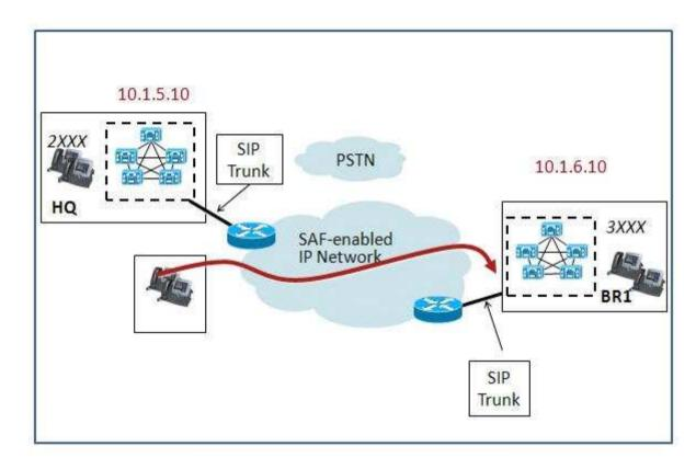
What should the destination IP address be configured as on the HQ and BR1 SIP trunks?
