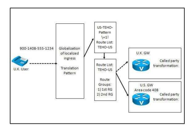
The exhibit shows centralized Cisco Unified Communications Manager configuration components for TEHO calls to U.S. area code 408 from the U.K. The PSTN access code for the U.K. is 9 and 001 for international calls to the U.S. What should the TEHO-US route list configuration consist of?
