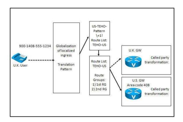
The exhibit shows centralized Cisco Unified Communications Manager configuration components for TEHO calls to U.S. area code 408 from the U.K. The PSTN access code for the U.K. is 9 and 001 for international calls to the U.S. To match the US-TEHO pattern \+!, how should the translation pattern be configured?
