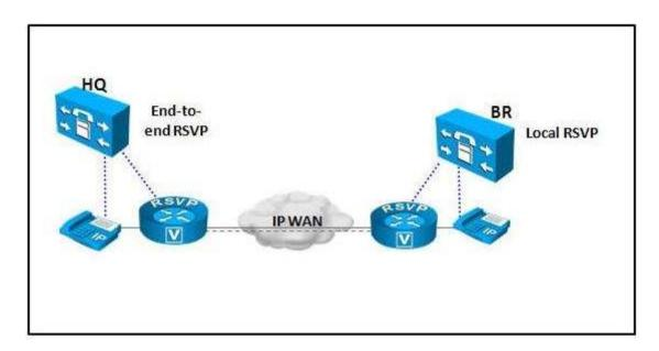
The HQ Cisco Unified Communications Manager has been configured for end-to-end RSVP. The BR Cisco Unified Communications Manager has been configured for local RSVP.
