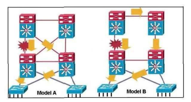
Model A is the recommended design for routing between Building Distribution switches and Campus Core switches. Which two statements describe the reasons? (Choose two)
