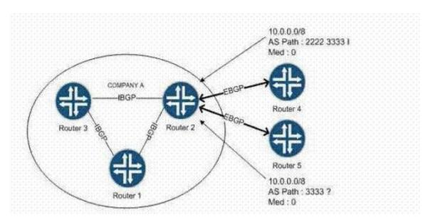
Router 2 is receiving a route to 10.0.0.0/8 from Router 4 and Router 5. What will Router 2 do with the routes shown in the exhibit?
