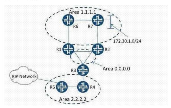
In the exhibit, Areas 1.1.1.1 and 2.2.2.2 are configured as normal areas. In R7's OSPF configuration, the interface on the 172.30.1.0/24 network is configured with the passive option. In which LSA type does R5 receive the announcement for the 172.30.1.0/24 network?
