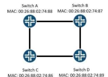
A network administrator has connected four switches as shown in the exhibit. The switches are at their factory-default configurations and the administrator powers on all of the switches at the same time. Which switch will become the root bridge?
