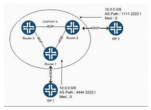
Router 2 is receiving two announcements of a route to 10.0.0.0/8. Router 2 learned one version of the route from ISP-2; this announcement of the route was received first. The second announcement of the route was received from Router 1 using IBGP. What will Router 2 do with the routes shown in the exhibit?
