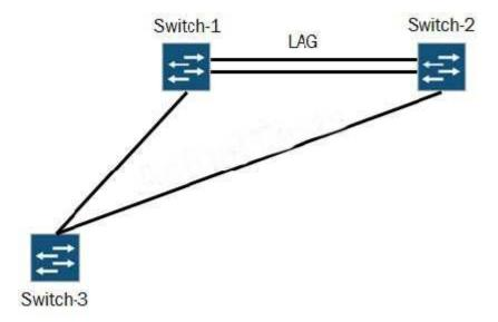
Referring to the exhibit, you want to avoid using STP and the LAG is configured on ae0. Which function would you use to prevent a Layer 2 loop?
