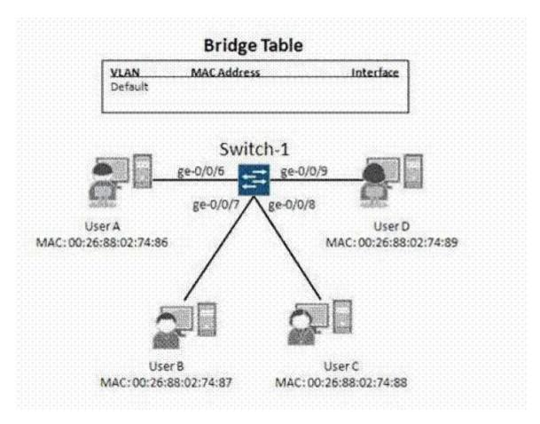
On Switch-1, all configured interfaces belong to the default VLAN. Based on the topology and bridge table shown in the exhibit, which two operations will Switch-1 perform if it receives a frame sent by User A with a destination MAC address of 00:26:88:02:74:89? (Choose two.)
