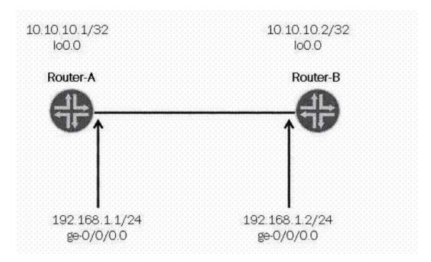
Router-A and Router-B shown in the exhibit are peering between their loopback interfaces. Which operational command on Router-A do you use to display all the BGP routes received from Router-B?
