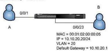
Referring to the exhibit, a packet sent from User A to User B will be forwarded out interface 0/0/23 using which source MAC address?
