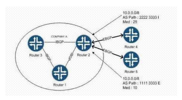
Router 2 is receiving a route to 10.0.0.0/8 from Router 4 and Router 5. What will Router 2 do with the routes shown in the exhibit?
