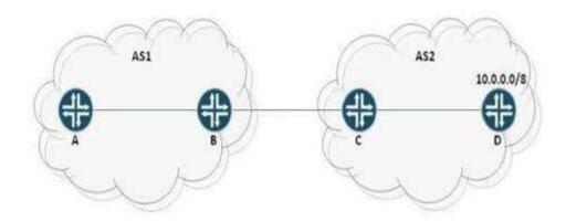
Router D is advertising a path for the 10.0.0.0/8 network through BGP and AS 2 is advertising this path to AS 1. By default, what is the next hop for this path from router A's perspective?
