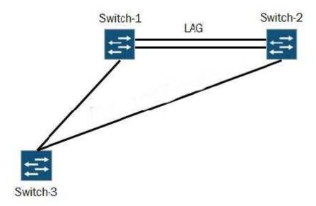
Your current network is using Switch-1 and Switch-2 as a Layer 3 core pair. You change the EX series switch core into a VC and configure the links between the switches to be a LAG. Assuming that Switch-3 is operating at Layer 2 only, which two protocols would be removed from this portion of the network? (Choose two.)
