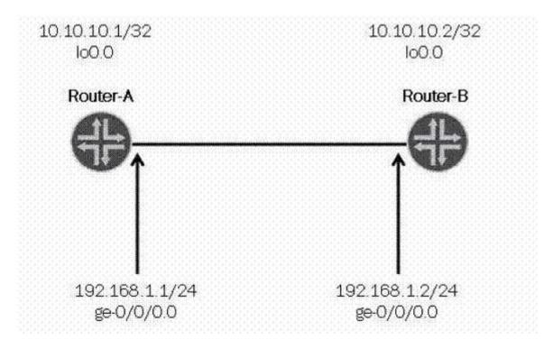
Router-A and Router-B shown in the exhibit are peering between their loopback interfaces. Which operational-mode command on Router-B do you use to display the BGP routes advertised to Router-A?
