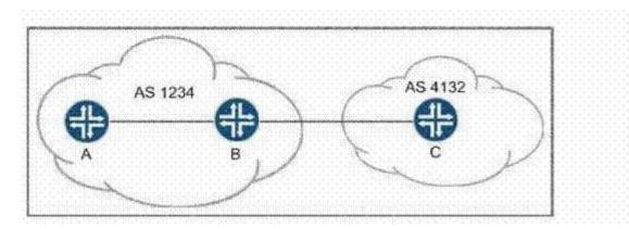
In the exhibit, the 172.32.1.0/24 prefix is being sent from Router A to Router B through BGP. When the BGP announcement for 172.23.1.0/24 is sent from Router B and received by Router C, which two attributes will be changed by default? (Choose two.)
