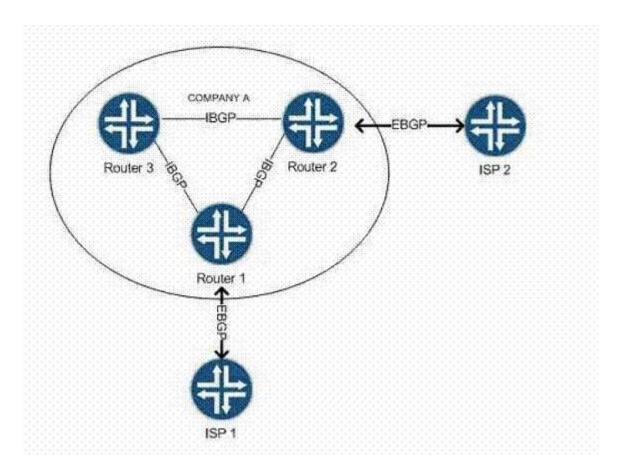
Company A wants to control how BGP traffic reaches the Internet. What should you configure to ensure that traffic exits the network by way of Router 1 toward ISP 1?
