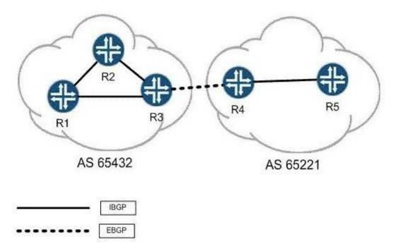
A route is advertised from AS 65221 to AS 65432 using EBGP. The route is active and reachable on R3, but does not appear as an active route on R1 and R2. R3 has an export policy applied to its IBGP group matching on routes from R4, but does not have a then criteria specified. Which policy action should router R3 configure to make this route visible on routers R1 and R2?
