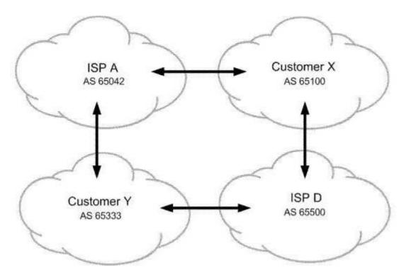
All ISP networks shown in the exhibit contain many BGP speaking routers. You are in charge of ISP A. You must ensure that customer Y sends their traffic to you over the directly connected link but customer Y is not used for transit into your network. What do you do to accomplish this?
