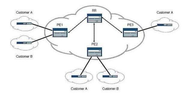
Referring to the exhibit, you want to save CPU processing load on the PE3 router by preventing the reception of routes belonging to Customer B. Which Layer 3 VPN scaling mechanism provides this functionality?
