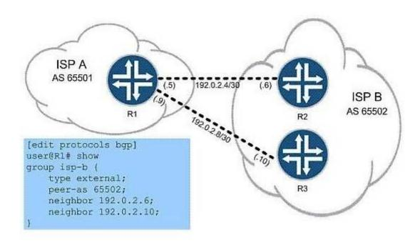
You work for ISP A, as shown in the exhibit, and must configure R1 to use load balancing across both available links for all routes to ISP B's network. You start by configuring this policy:
