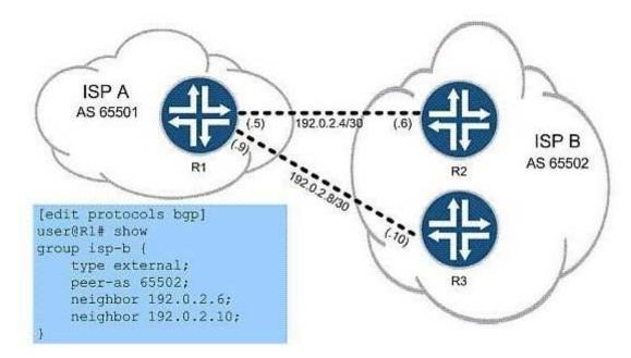
Referring to the exhibit, you work for ISP A and are asked to configure R1 to forward traffic for all routes across both available links, to both routers in ISP B's network. Which three configuration commands do you use? (Choose three.)
