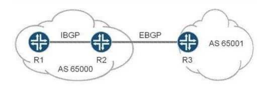
The exhibit contains a BGP topology. R1 and R2 are peering using IBGP. R2 and R3 are peering with EBGP. R1 is not installing any routes from R3 due to next-hop resolution issues. Which two configurations will resolve this issue? (Choose two.)
