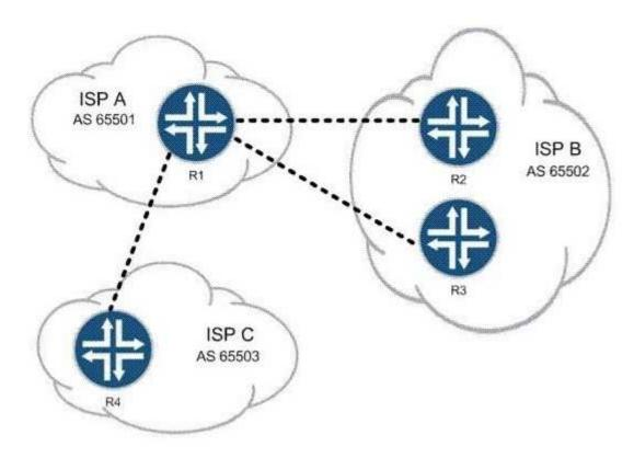
You work for ISP A. Customers of both ISP B and ISP C must be able to reach all of your customers, but your network must not allow transit traffic between ISP B and ISP C. Referring to the exhibit, which two methods could you use? (Choose two.)
