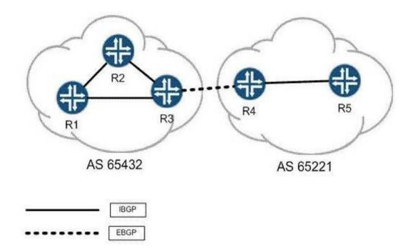
R3 and R4 want to establish an EBGP session between each other's loopback addresses. They have each configured static routes to the other's loopback address and can ping from loopback to loopback. Their EBGP session is configured with correct neighbor and local addresses. The correct AS numbers have been specified at the [routing-options] hierarchy as well. Considering the topology in the exhibit, which statement is true?
