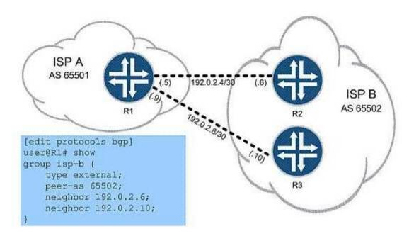
You work for ISP A, as shown in the exhibit, and must configure R1 to use load balancing across both available links to ISP B's network. Which command do you use to finish the configuration?
