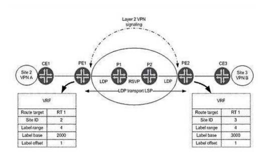
In the exhibit, on which label value does PE1 expect to receive traffic from CE3 for VPN A?
