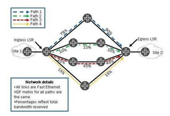
You have an MPLS network and you have configured most-fill as a CSPF tiebreaker. Using the information in the exhibit, which path will be used to signal a new LSP requiring 12 Mbps?
