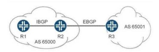
The exhibit contains a BGP topology. R1 and R2 are peering using IBGP. R2 and R3 are peering with EBGP. R1 is not installing any routes from R3 due to next-hop resolution issues. Which two configurations will resolve this issue? (Choose two.)
