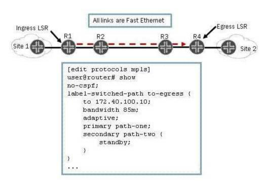
As shown in the exhibit, you have an adaptive LSP that requires 85 Mbps. The LSP is configured with a primary path and a secondary path in standby mode. All connections in the MPLS network are Fast Ethernet. Which statement is correct?
