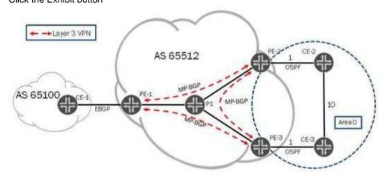
You manage the network in the exhibit. Your customer contacts you and requests that OSPF traffic being routed between CE-2 and CE-3 use the VPN connection instead of the direct connection in its local network.
