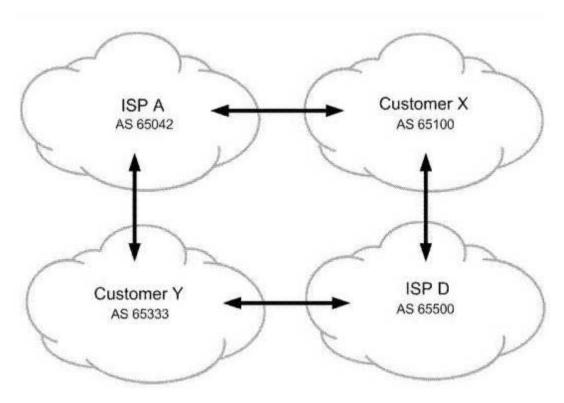
All networks shown in the exhibit contain more than one BGP speaking router. You operate ISP A. You must ensure that customer Y sends their traffic to you over the directly connected link but customer Y is not used for transit into your network. What do you do to accomplish this?
