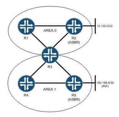
You are asked to configure an OSPF network based on the topology shown in the exhibit. Area 1 must not receive Type 5 LSAs from the backbone, but must be capable of containing ASBRs. What will accomplish this?
