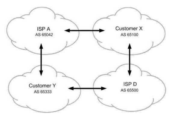
All ISP networks shown in the exhibit contain many BGP speaking routers. You are in charge of ISP A. You must ensure that customer Y sends their traffic to you over the directly connected link but customer Y is not used for transit into your network. What do you do to accomplish this?
