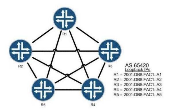
All routers shown in the exhibit are BGP neighbors. R1 must be a route reflector, and R2 through R5 must be clients. R2 should only receive one copy of all routes sent from R4.Which configuration is valid?
