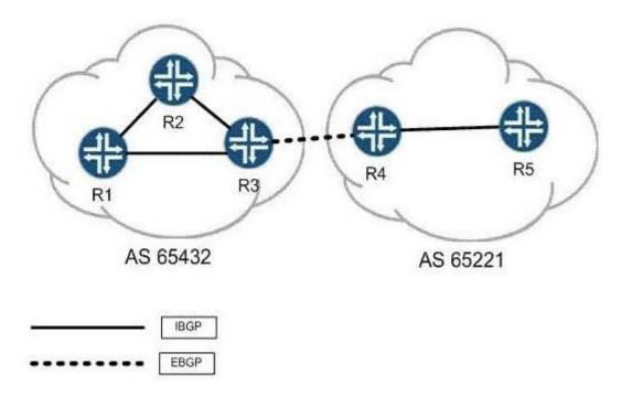
R3 and R4 want to establish an EBGP session between each other's loopback addresses. They have each configured static routes to the other's loopback address and can ping from loopback to loopback. Their EBGP session is configured with correct neighbor and local addresses. The
