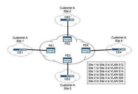
You are provisioning a full-mesh BGP Layer 2 VPN for Customer A. The customer has four remote sites in their network. Using best practices, you assigned interface unit numbers matching the assigned VLAN numbers. Which Layer 2 VPN configuration is correct for PE2?
