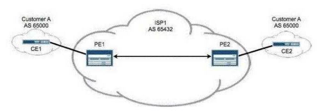
In the exhibit, your Layer 3 VPN uses BGP to send and receive routes from customers. Customer A reports that remote routes are not being received on CE2. Which configuration parameter is missing from your PE router configuration?
