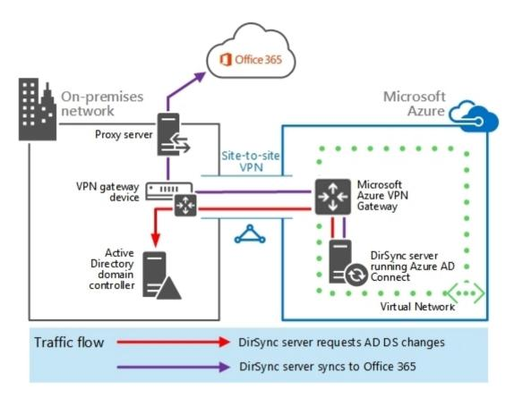
Azure AD Connect tool on a virtual machine in Azure synchronizing on-premises accounts to the Azure AD tenant of an Office 365 subscription with traffic flow.
