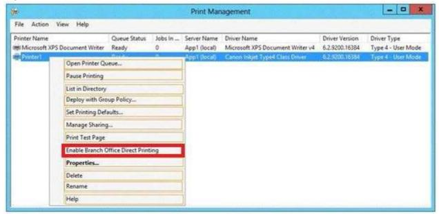
Branch Office Direct Printing can reduce Wide Area Network (WAN) usage by printing directly to a print device instead of a server print queue. This feature can be enabled or disabled on a per printer basis and is transparent to the user.
