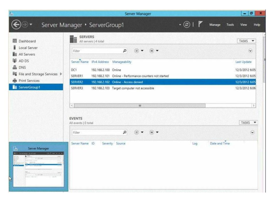
You need to ensure that Server2 can be managed remotely by using Server Manager.
