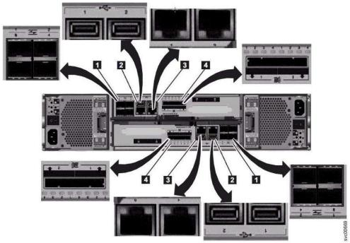
Using the diagram as a reference, what number refers to where the USB key can be inserted?
